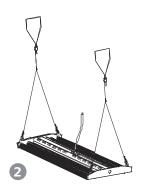
STEP TWO Connect ropes with high bay properly and make sure the high bay is hanging straightly
