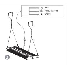
STEP THREE Install the high bay to needed position solidly and finish wiring according to instruction.
